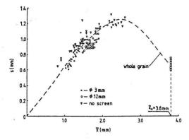
Fig. 3. The relationship of the particle mean size  $\overline{x}$  and the standard deviation s with barley grinds.
