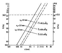
Fig. 1. Typical Rosin-Rammler distributions on RRSBnet, while n=const. and  $x_0$  parameter varies.
