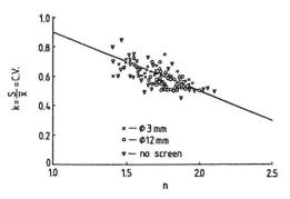
Fig. 4. The relationship of the coefficient of variation C.V. and Rosin-Rammler's uniformity coefficient n with barley grinds.
